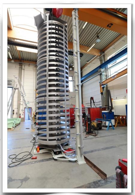
Since I was helping Halil in the process of aligning the water cooling spine and spiral conveyor, I could not take a picture before the **L** was welded but managed to take one after we had attached the first water inlet pipe between the water cooling spine and the spiral conveyor.
