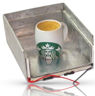
Thermoelectric Cooler (TEC): Thermoelectric coolers are "Solid State Heat Pumps" which work on the basis of Peltier Effect. When a
