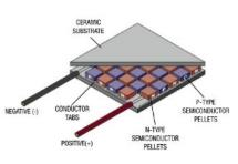
to use the difference in temperature of the cold and hot sides of thermocouple to generate enough voltage and current. Since I could not find any cheap source for Thermoelectric generators I thought why not try to use a Thermo-electric Cooler (see image) instead.
