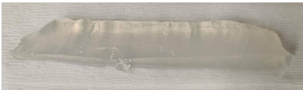
Figure 4: Salted Gelatin with a dielectric close to that of the eel's body.
